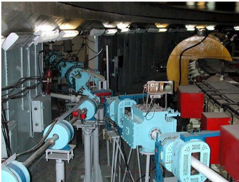
Fig.2. View of beamline of 75 MeV injector-linac (right beamline) and 20 MeV deflected beamline (left beamline)
