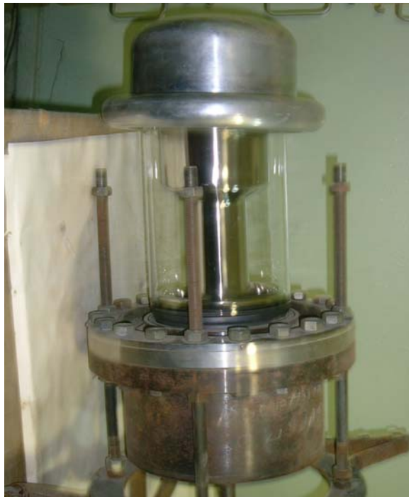
Fig.1. electron gun with 150 keV, 10 A parameters
